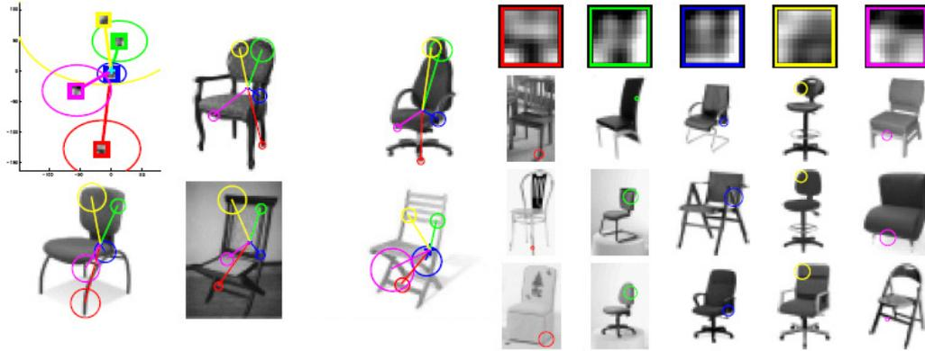
Figure 7: 5 parts from a chair model. The model is presented in the same format as Figure 6. Model parts represent the tip of the chairs leg(first part), edges of the back (second and fourth parts), the seat corner(third) and the seat edge(fifth). The location model is exaggerated: The tip of the chairs leg is modeled as being far below its real mean position in object images.
