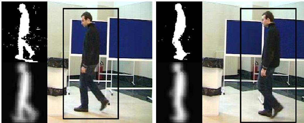
Figure 5. Application of the proposed silhouette based tracking approach on a publicly available video sequence, from which two frames are shown. The background subtracted image and the best corresponding shape in the model are depicted on the left.
