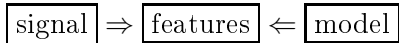
Figure 1: The traditional ‘forward’ approach to feature extraction and modelling. First features are extracted from the signal which are subsequently modelled, p(\text{features}|\text{signal}, \text{model}) . Noise effects are dealt with by choosing appropriate features which are as ‘noise’ free as possible.
