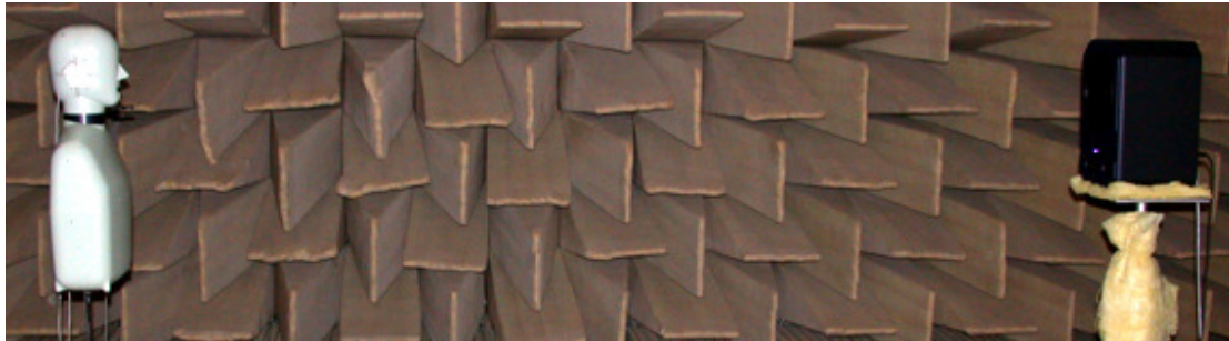
Figure 4. Setup for impulse response measurement in the anechoic chamber.
