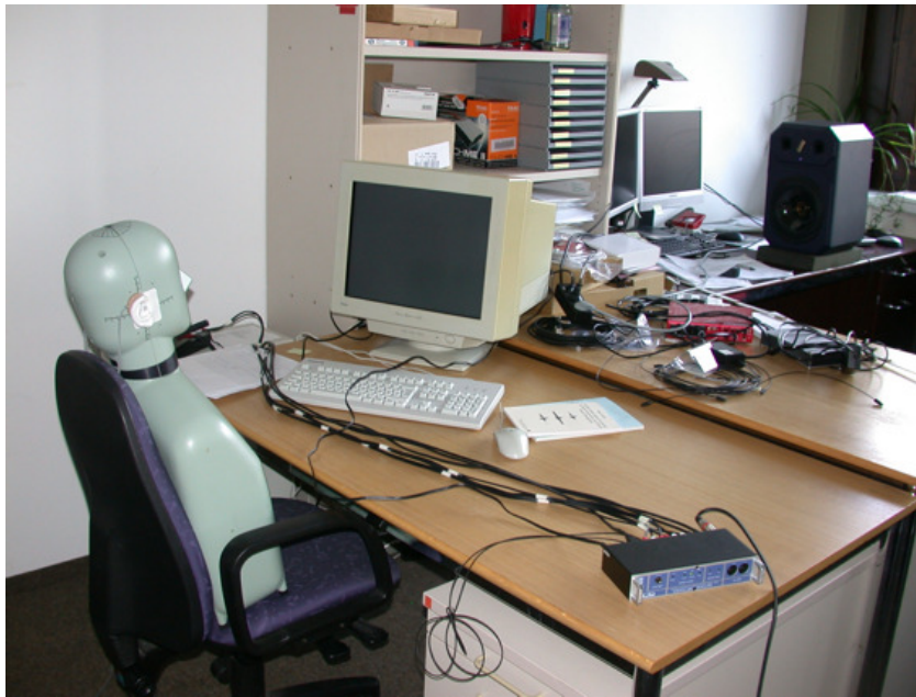
Figure 6. Office at the University of Oldenburg where recordings were performed, showing the head and torso simulator with recording equipment.
